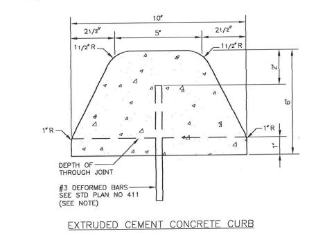
NOTE: ALTERNATELY, THE USE OF EPOXY BONDING AGENT, IN PLACE OF #3 DEFORMED BARS, WILL BE ALLOWED.
