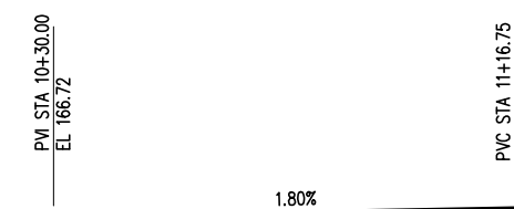
N-LINE PROFILE AT BRIDGE
