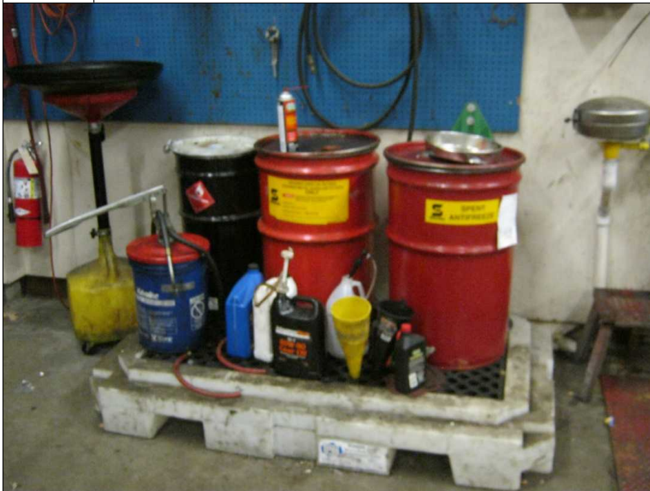
12. Waste automotive fluids on secondary containment
