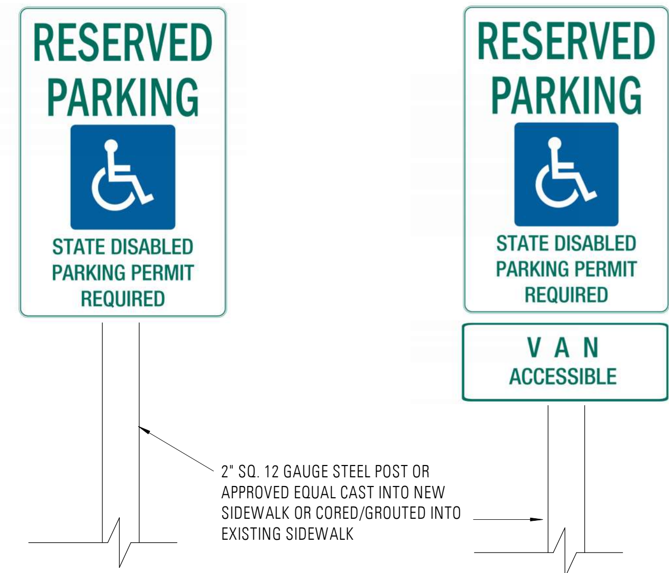
DETAIL - ADA SIGNAGE NOT TO SCALE
